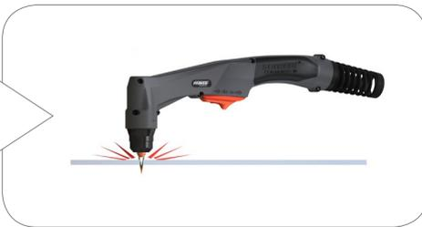
If sparks are spraying up from the workpiece, you are moving the torch too fast, or without sufficient power.
