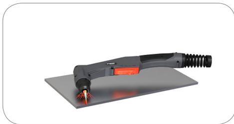
Hold the torch at a 45° angle to the workpiece. Pull the trigger to obtain a pilot arc. Transfer the arc to the work piece.
