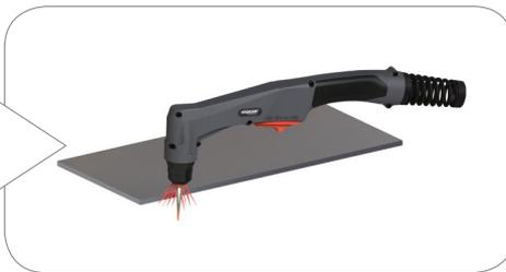
Pull the trigger to start the pilot arc. The cutting arc will initiate when the torch parts are in the correct proximity to the workpiece. Start cutting at the edge until the arc has completely cut through the workpiece.
