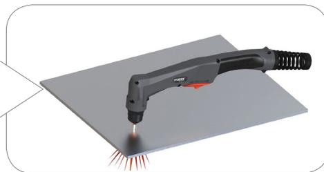
When sparks are exiting from the bottom of the workpiece, the arc has pierced through the material.
