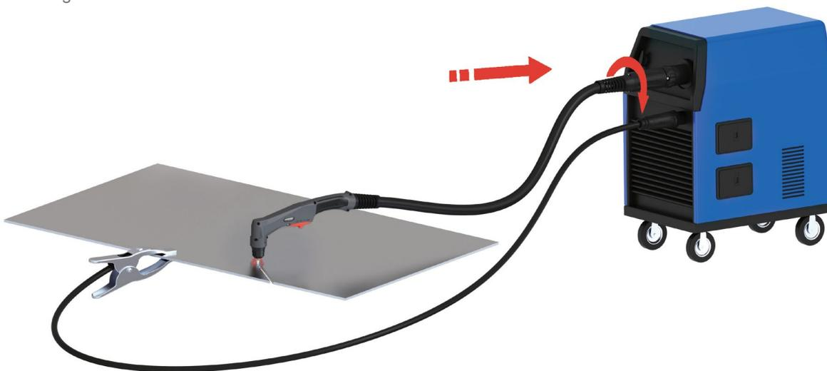
Attach the work clamp securely to the workpiece. Remove rust, paint or other coatings to ensure good electrical contact. Attach the work clamp as close as possible to the area being cut, to reduce exposure to electromagnetic fields (EMF).
