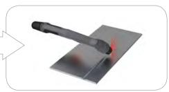
Maintain an approximate 45° angle to the workpiece. Feed into the gouge.
