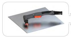
Fire the torch at an angle to the workpiece, then slowly rotate it to an upright position.
