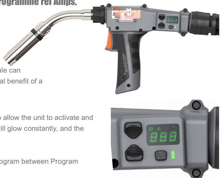
The selected function can then be changed by holding down either the upper finger pad to increase or the lower finger pad to decrease. Once set, the unit can be de-activated by switching it off by pressing and holding the mode switch (M). This will prevent accidental changes to the chosen settings during the welding operation. When re-activated, the unit returns to the current setting.
